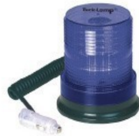
JBM62VB 60 LED Blue Light 360° Flasher Magnetic Mount 120x123mm 10-30v
