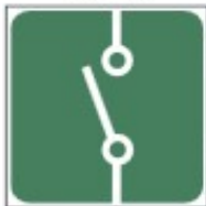
Electric Isolator Switch
