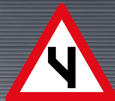
W119: Beginning of Dual Roadway Sign
