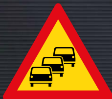
TW355: Congestion Sign
