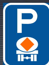
R316-P: Vehicle Conveying Dangerous Substances Parking Reservation Sign
