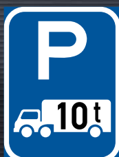
R314-P: Goods Vehicle Exceeding Indicated GVM Parking Reservation Sign
