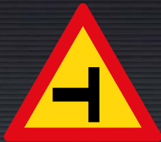
TW107: Left Side Road Junction Sign
