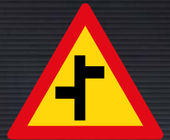
TW110: Staggered Junction Sign
