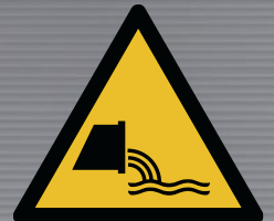
W055 sewage effluent outfall
