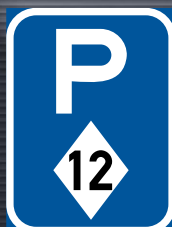
R320-P: High Occupancy Vehicle Parking Reservation Sign
