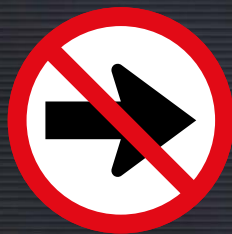
R212: Right Turn Prohibited Sign
