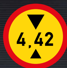
TR204: Height Limit Sign
