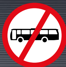
R227: Buses Prohibited Sign
