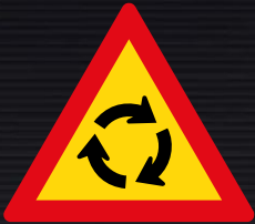
TW201: Traffic Circle Sign
