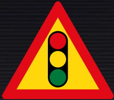
TW301: Traffic Signal Ahead Sign
