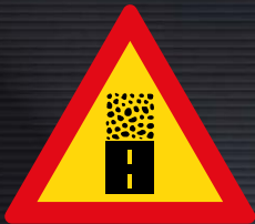
TW325: Gravel Road Begins Ahead Sign
