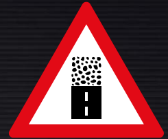
W325: Gravel Road Begins Ahead Sign
