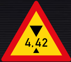
TW320: Height Restriction Sign
