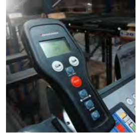
Operation of the shuttle via handheld radio terminal.
