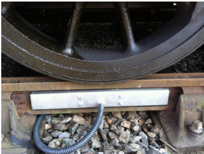
Load cells under each wheel to be weighed.
