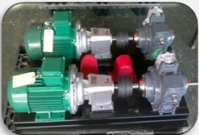
Electrical Motor Pump Skid
