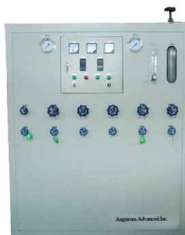
D. Hydrogen Generating Plant by Pressure Swing Adsorption with H 2 Purifying
