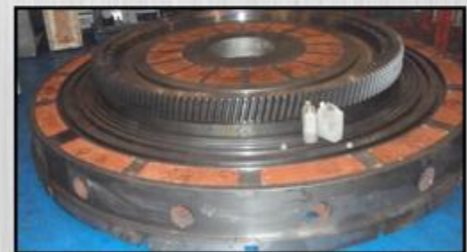
EXTRA HEAVY DUTY DOUBLE ROW HYDROSTATIC BEARING
