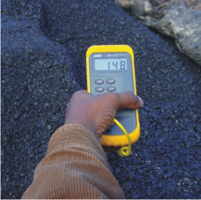
Testing the temperature of the mix using a digital probe thermometer
