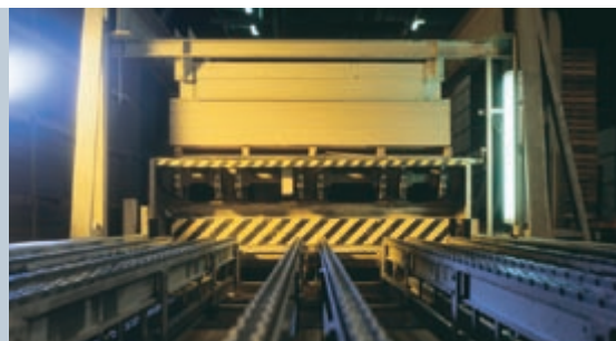
A finished raw panel exits the dryer
